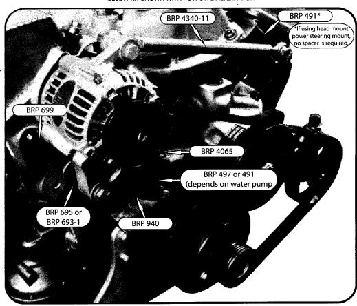
PLEASE NOTE: DUE TO VARIATIONS IN WATER PUMP AND ALTERNATOR MOUNTING, SPACER CONFIGURATIONS MAY NEED TO BE CHANGED. ONLY USE THIS SHEET AS A GUIDE. SOME SPACERS MAY BE LEFT OVER AT THE END OF THIS INSTALLATION.
